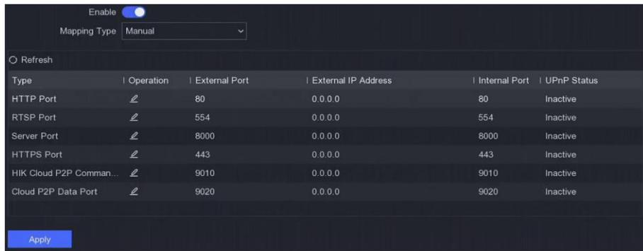
The screenshot shows a table of port mappings. The columns are Type, Operation, External Port, External IP Address, Internal Port, and UPnP Status. The rows include HTTP Port (80), RTSP Port (554), Server Port (8000), HTTPS Port (443), HIK Cloud P2P Command Port (9010), and Cloud P2P Data Port (9020). All ports are currently inactive.
