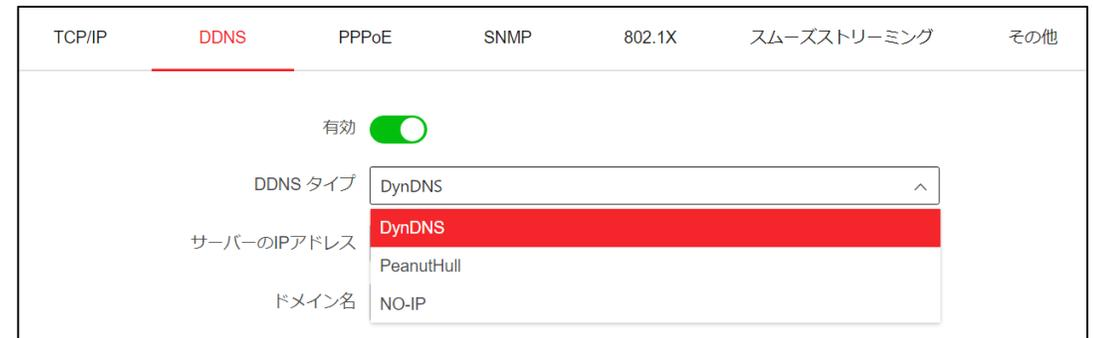
The screenshot shows the DDNS configuration page in an NVR interface. The page has a navigation bar at the top with tabs for TCP/IP, DDNS (selected), PPPoE, SNMP, 802.1X, スムーズストリーミング, and その他. Below the navigation bar, there is a toggle switch for '有効' (Enabled) which is turned on. Underneath, there are three labels: 'DDNS タイプ', 'サーバーのIPアドレス', and 'ドメイン名'. The 'DDNS タイプ' dropdown menu is open, showing three options: 'DynDNS' (highlighted in red), 'PeanutHull', and 'NO-IP'.
